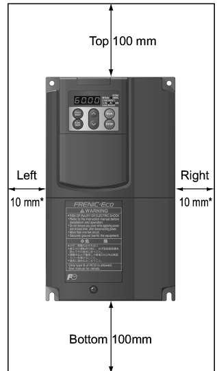
Figure 2.1 Mounting Direction and Required Clearances
